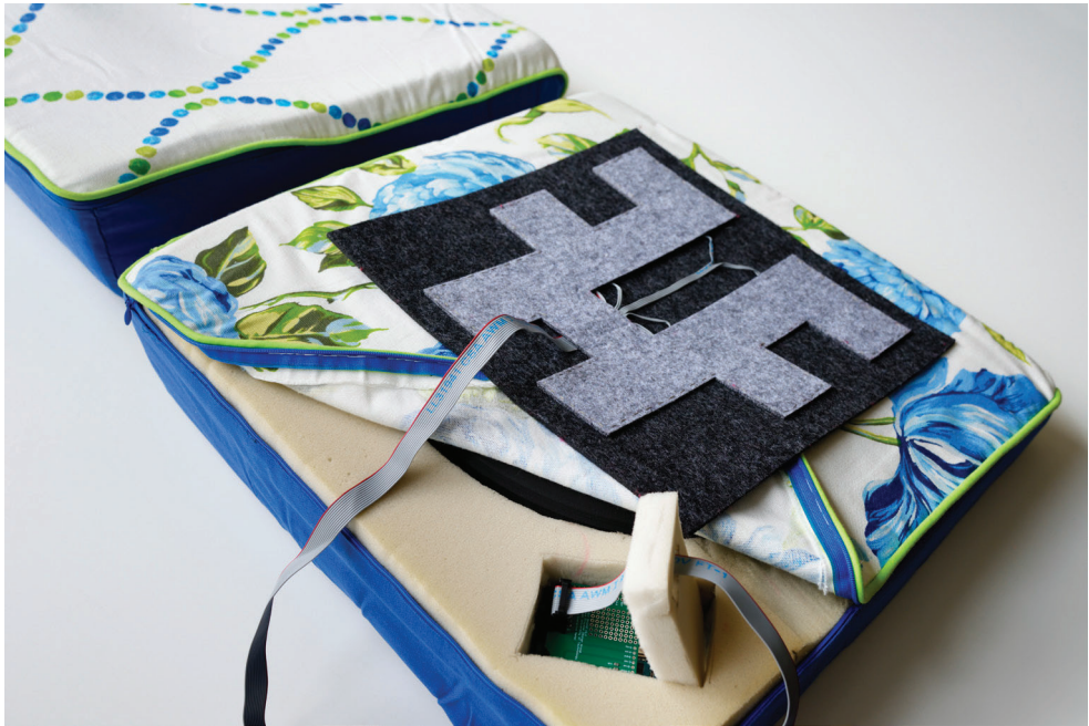
Figure 12: HealthSit active sitting sensor mat
